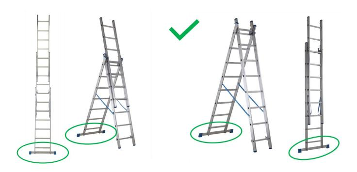
Always ensure that the bottom stabiliser bar is fitted correctly before any use. Failure to follow this set up could result in collapse of the ladder and possible serious injury.
