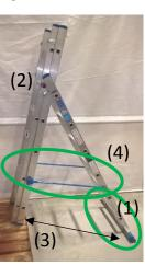
(1) Ensure the bottom stabiliser bar is fitted correctly before any use.
